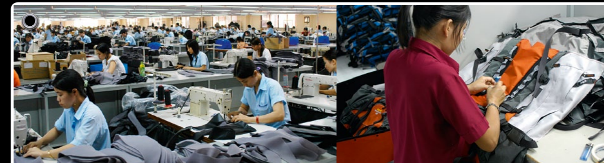
In spite of the most modern technology available, the majority of rucksack production is still done by hand. On 32 production lines, the 2,800 employees assemble as many as 221 components that can go into making a Deuter product.
